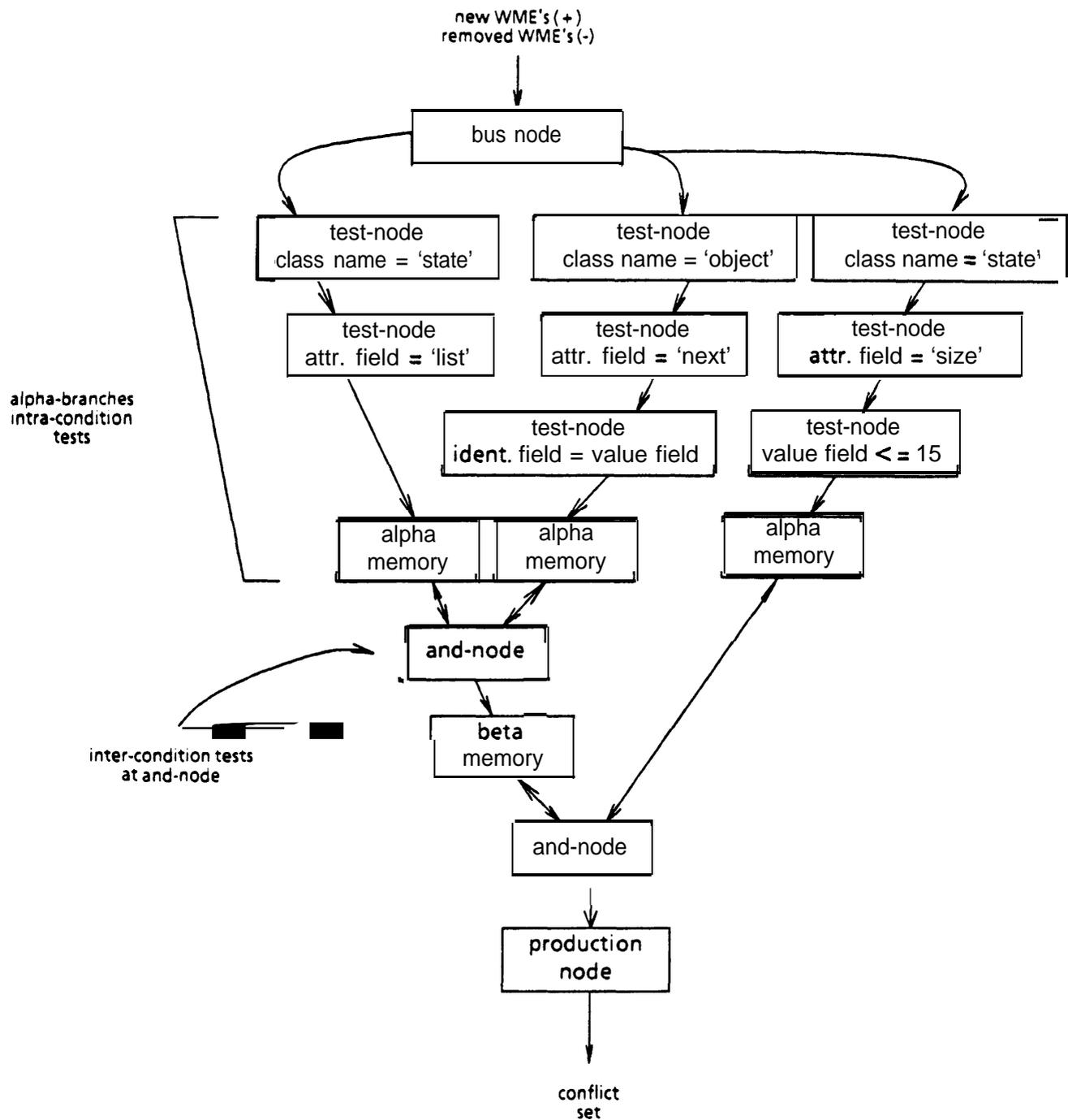
**Figure 4- 1:** Structure of a Small Rete Network
